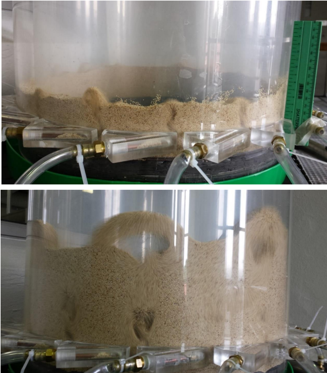
Figure 4-11: ( Top ) Jet formation (1.0 kg poppy seeds); ( bottom ) turbulent fluidization (2.0 kg poppy seeds)
