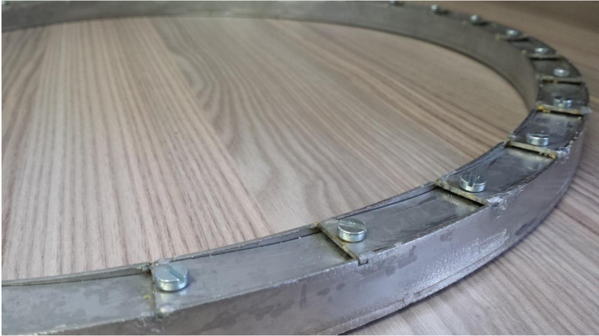
Figure 5-2: Photograph of the metal air distributor
