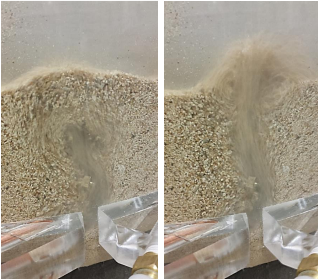
Figure 4-7: Instantaneous snapshots of jet formation (3.5 kg river sand)
