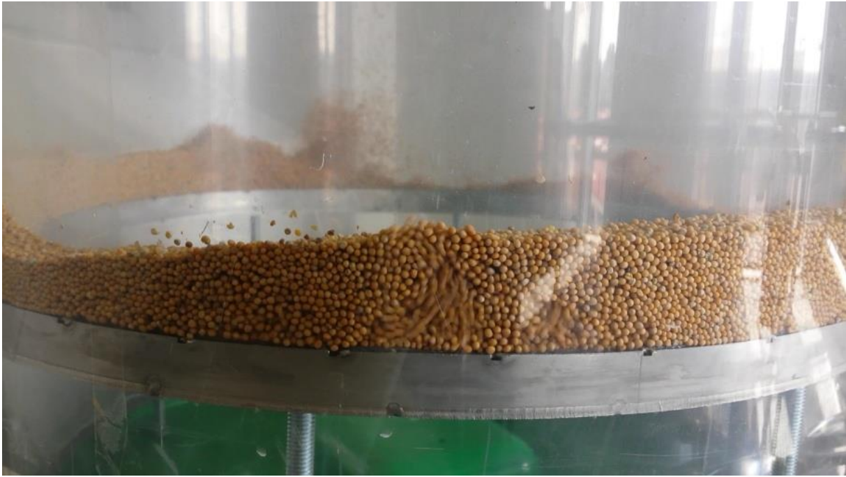
Figure 5-3: Seepage of fluidizing air along the inner walls of the Perspex tubes (0.5 kg mustard seeds)
