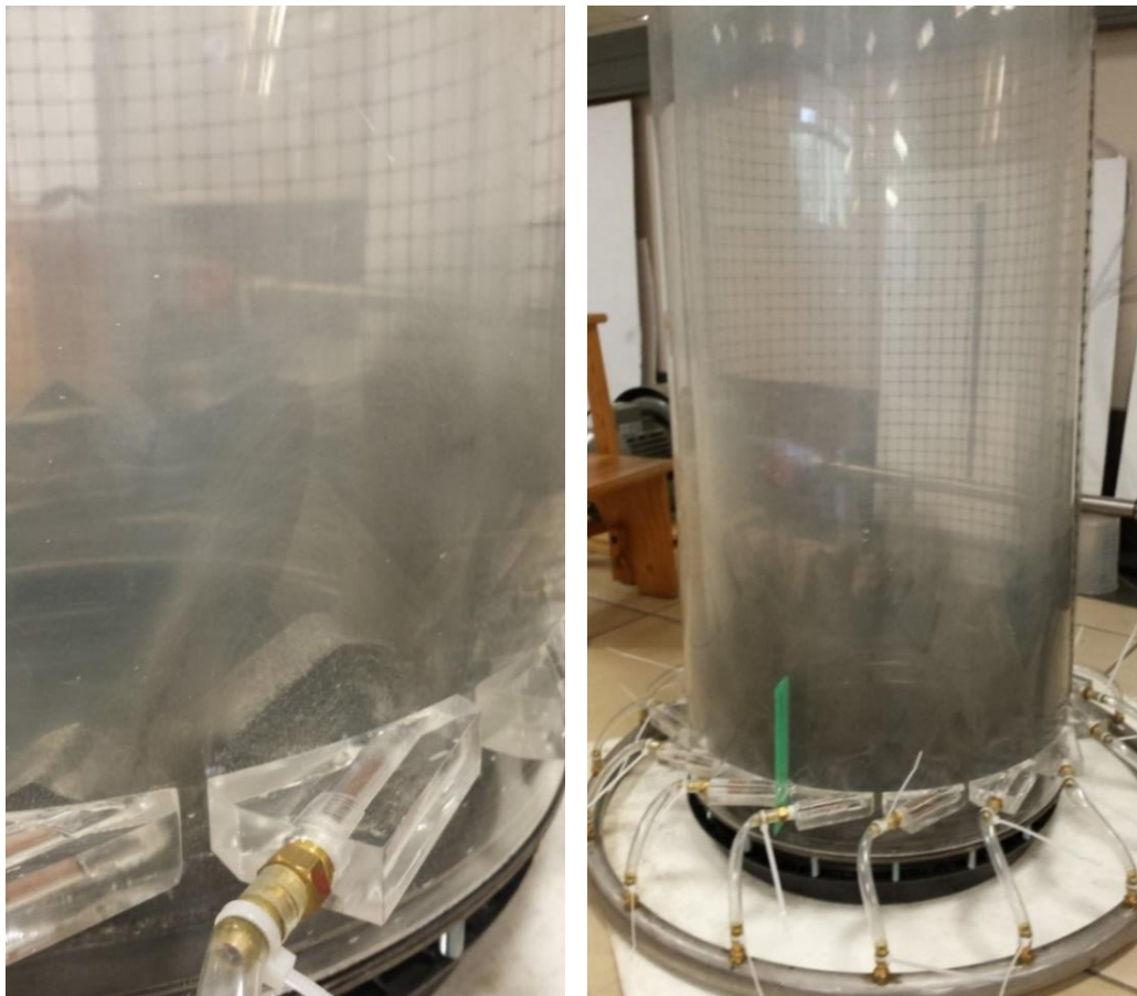
Figure 4-8: ( Left ) Depletion of bed material at several air injectors (3.0 kg ilmenite-sand mixture); ( right ) turbulent fluidization (4.0 kg ilmenite-sand mixture)
