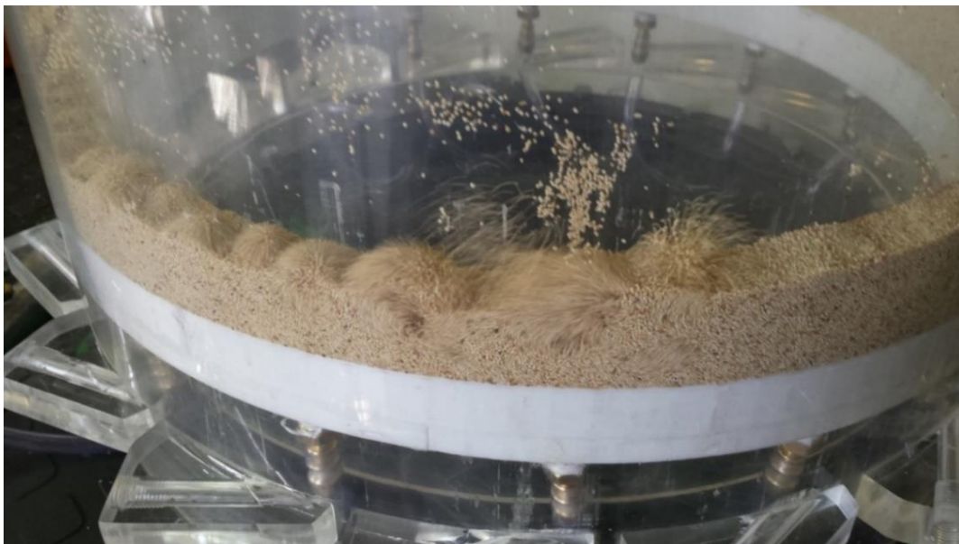
Figure 5-6: Bubbling fluidization behaviour (0.5 kg poppy seeds)
