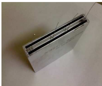
Figure 4 Brazed Test Unit
