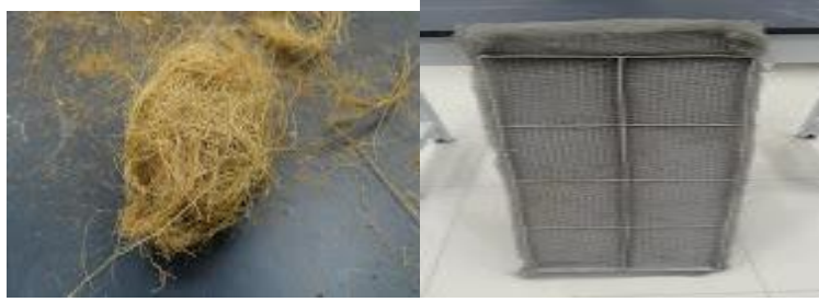
Figure 6. The date palm lufa and the stainless steel demisters.
