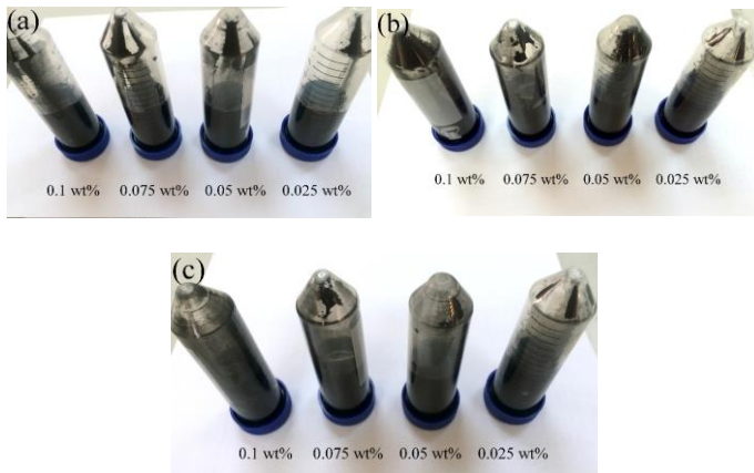
Figure 3 Visual investigation of sedimentation of nanofluids at 6000 rpm for three centrifugation times: (a) 5 min, (b) 10 min, (c) 20 min. Little sedimentation is observed on the bottoms of test tubes for all cases examined.
