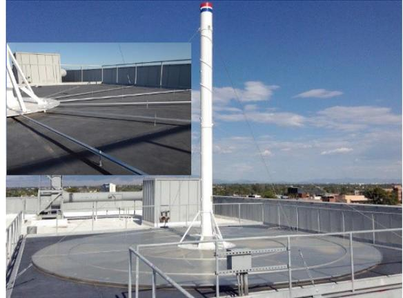
**Figure 1** 1:33 scale model of the Manzanares Solar Chimney Power Plant on the roof of the AME Building at the University of Arizona
