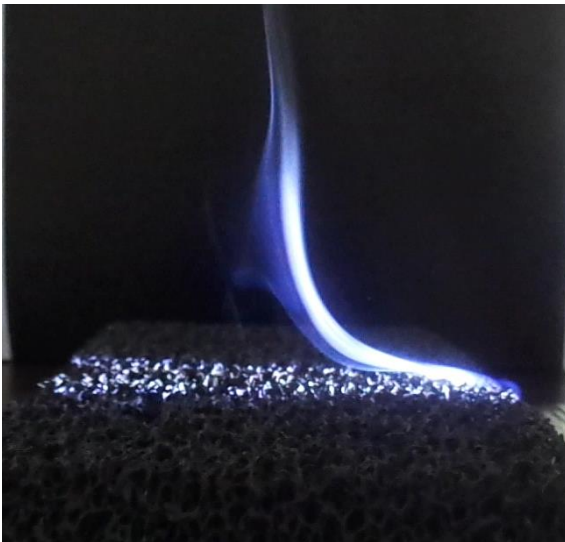
Figure 5 The deflection of the flow above the low painted metal foam heat sink in horizontal orientation.
