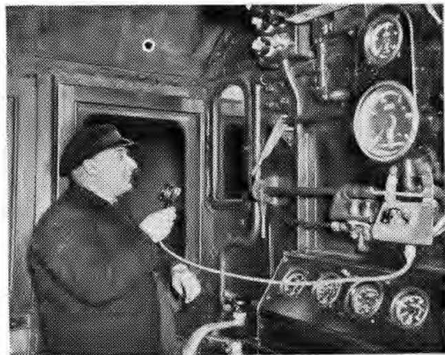
Radio-telephony control for locomotives, now being tried out on the British Railways.
