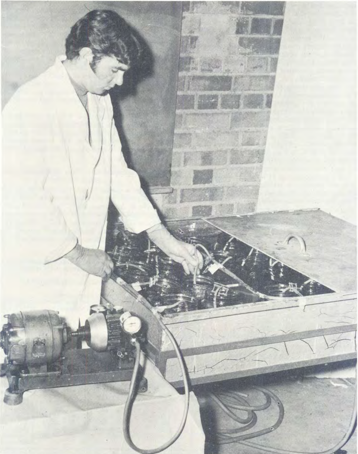
FIG. 1 The aeration apparatus for mixing the digests in the small waterbath
