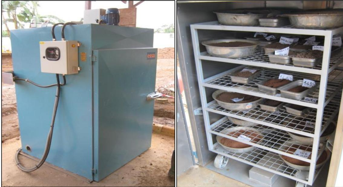
**Figure 4-17** Drying oven (*left*) and samples being dried (*right*)
