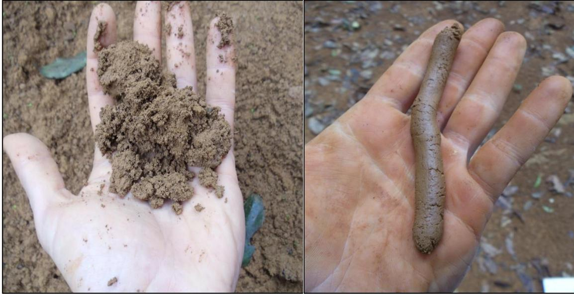
**Figure 4-19** Evaluating the material plasticity in the field during the site investigation
