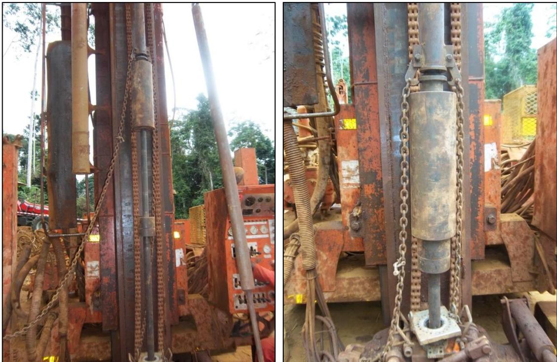
**Figure 4-15** SPT Apparatus used during geotechnical drilling
