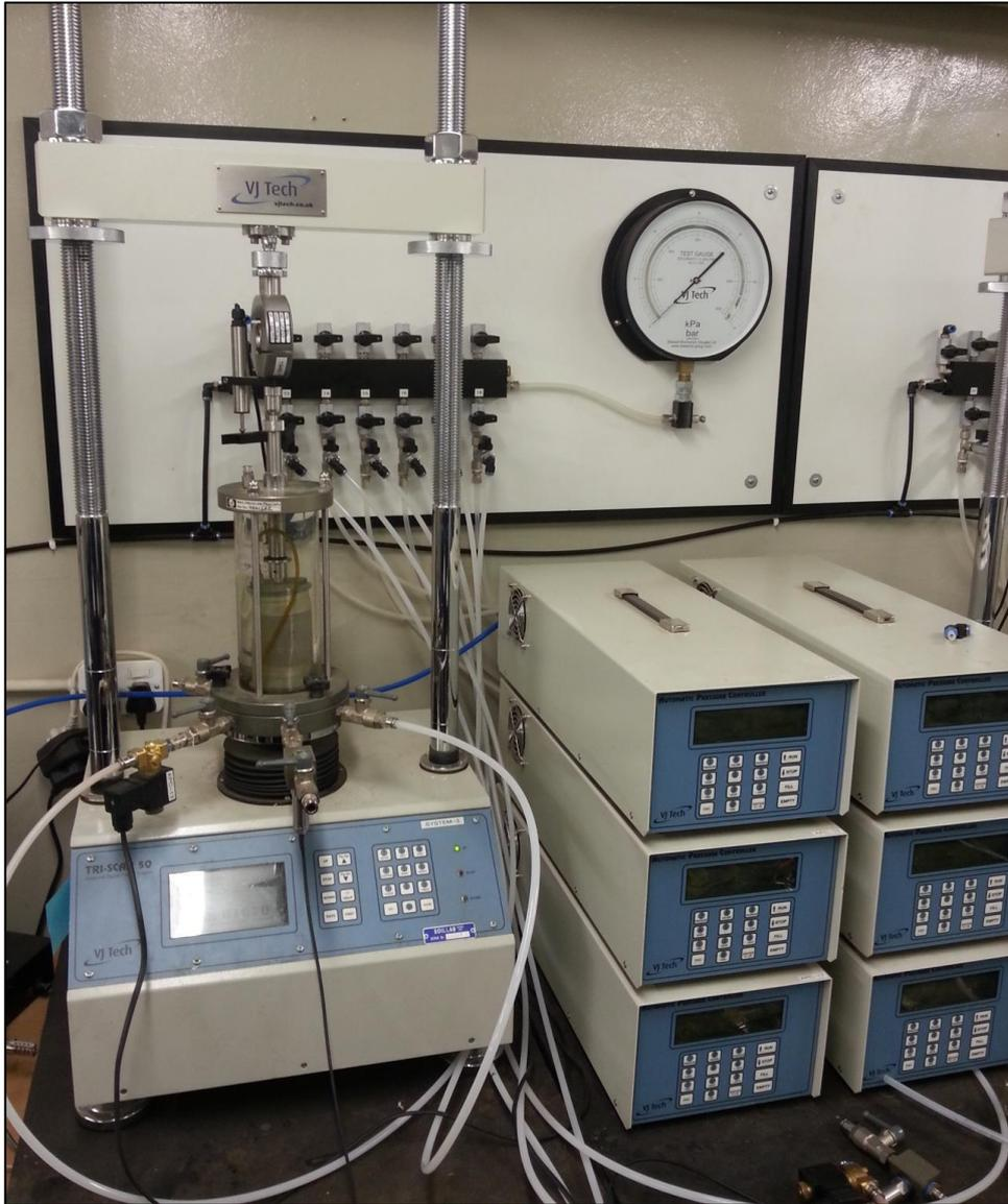
**Figure 4-22** Tri-axial apparatus setup maintained during research
