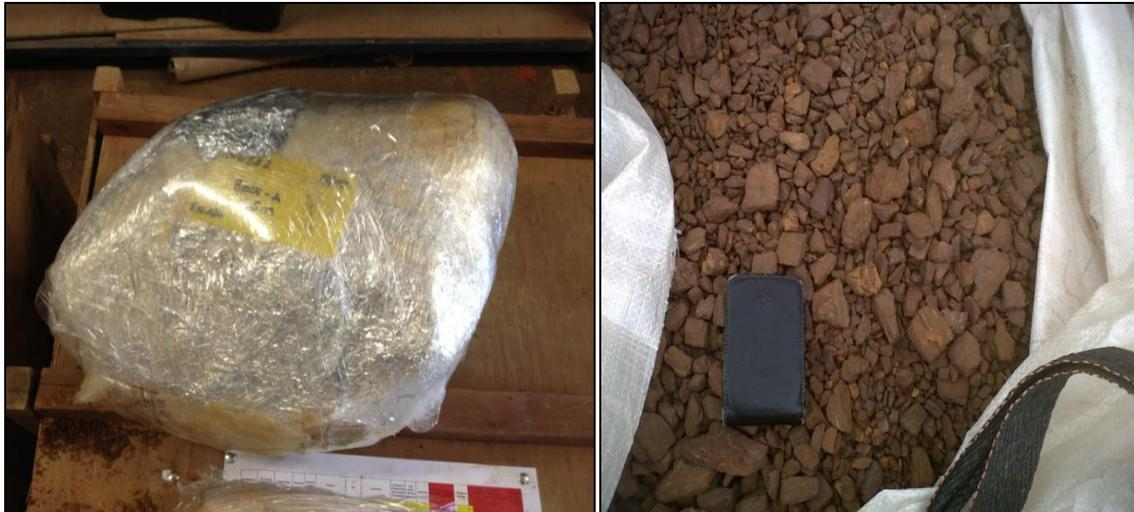
**Figure 4-9** Example of undisturbed sample (*left*) and bulk disturbed sample (*right*), both collected from the mining area
