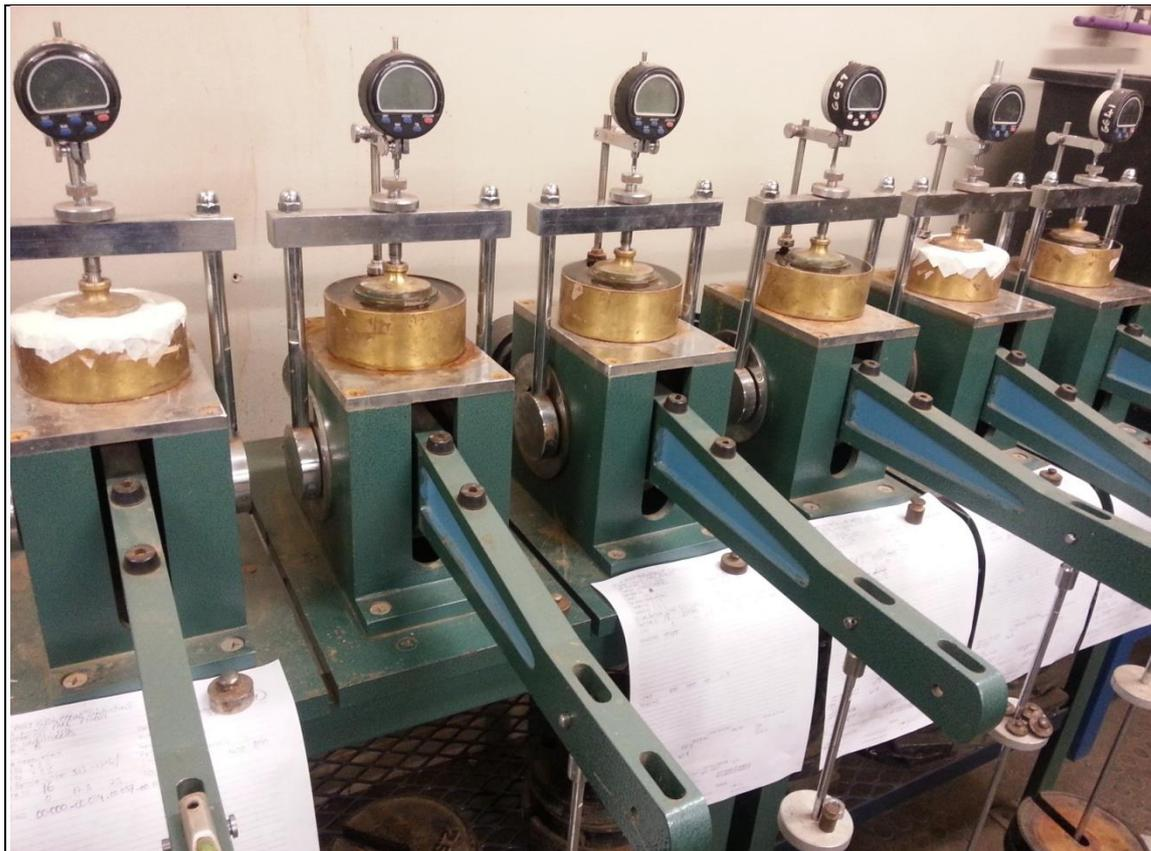
**Figure 4-24** Front loading Gang consolidometers during testing
