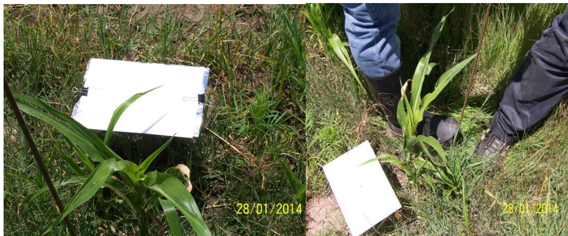
Figure 4.4 Chromatography paper (27 × 15 cm) mounted 20 cm above the ground and held in place with clips on an aluminium surface for spray drift deposition sampling.
