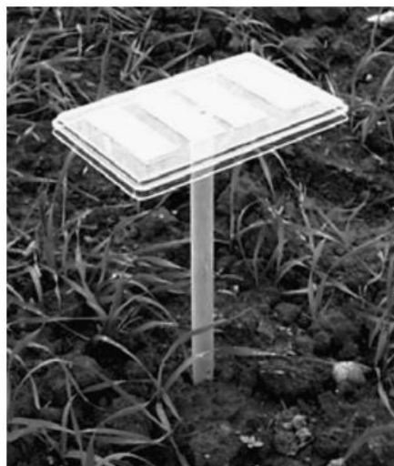
Figure 2.4 A passive dosimeter for collecting pesticide spray drift. It consists of four microscope slides placed on a plastic lid which is then mounted about 20 cm above ground (Carlsen et al. , 2006a).
