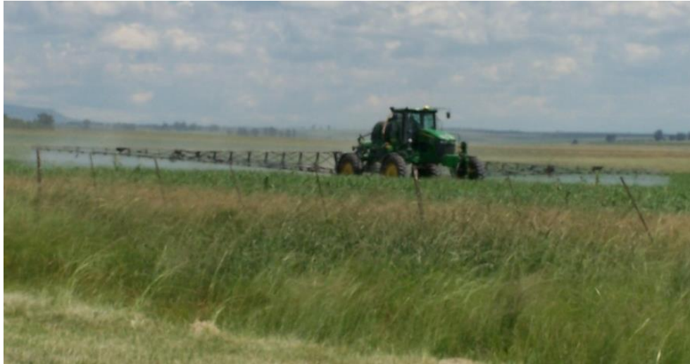
Figure 4.1 The "Tall-boy" ground sprayer used for pesticide application. The sprayer had a 32 m wide boom on which 56 TwinJet nozzles were distributed.
