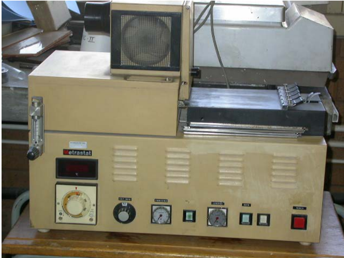
Metrastat thermal stability oven used during this research
