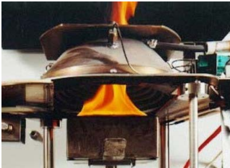
One-dimensional burning model Detail of the cone calorimeter set-up
