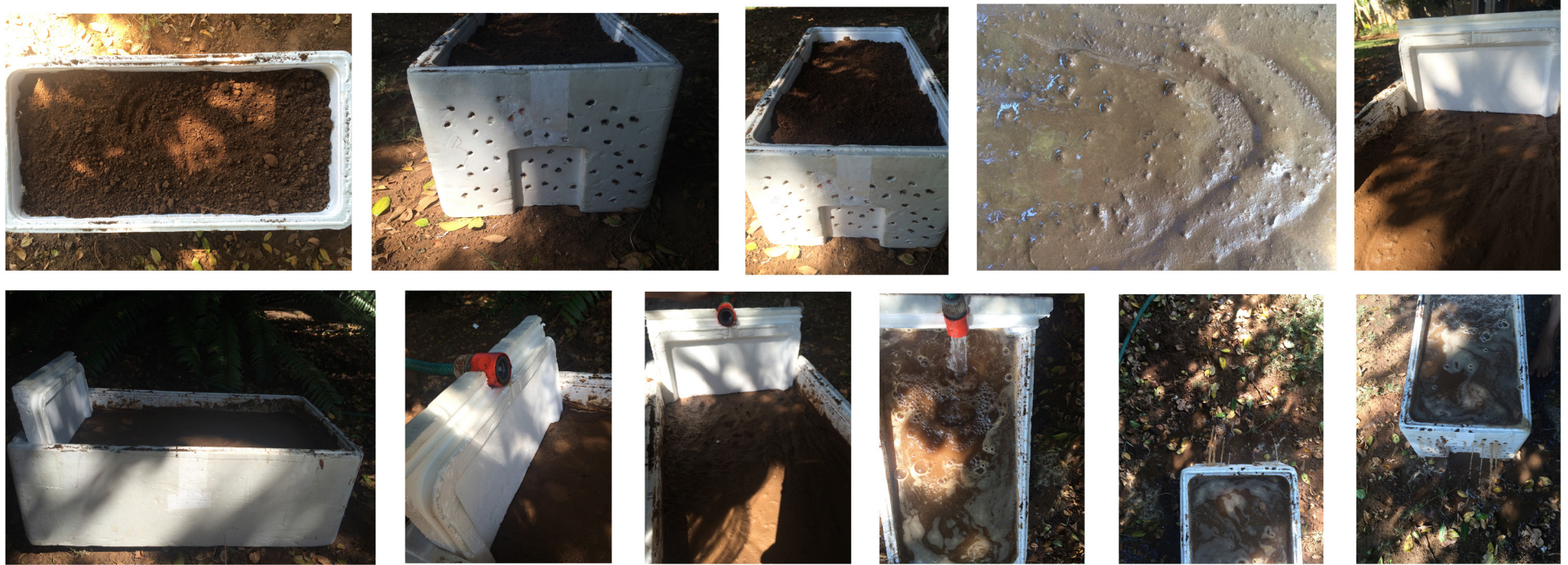
Experimenting with the effects of water on exposed soil. This experiment was done with the design in mind that where the dam wall overflows, it can be left to carve away soil, showing the forces of nature that influences the landscape forms.
