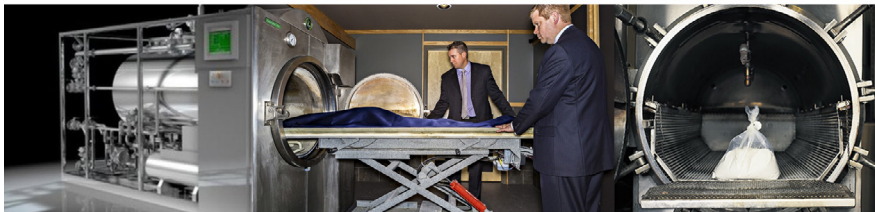
Figure 9. Resomator used for resomation of a corpse (Davies & Rumble 2012).
