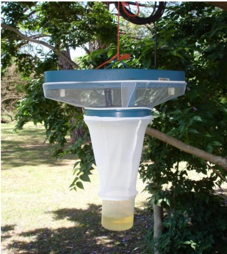
Figure 7: 220V Onderstepoort downdraft suction light traps with collection container (ARC-Institute of Agricultural Engineering, South Africa). © G.J. Venter.
