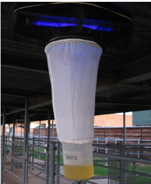
Figure 2. Onderstepoort suction light trap fitted with alphacypermethrin-treated HDPE mesh.
