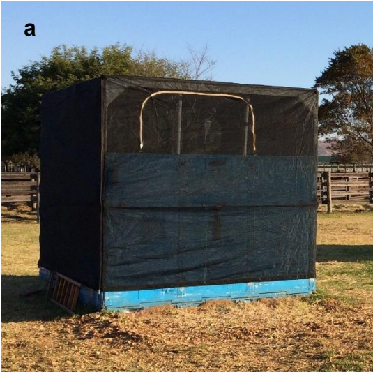
Figure 9. Jet stall protected with alphacypermethrin-treated HDPE mesh (a) and untreated jet stall (b).
