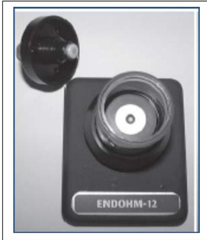
Figure 5.1. Endohm chamber used to measure TEER.
