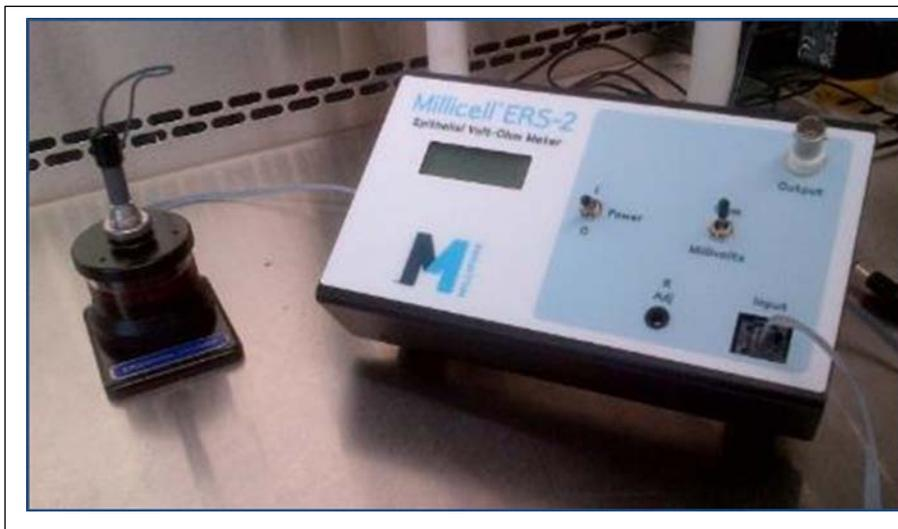
Figure 5.2. Volt-Ohm meter used to measure TEER.
