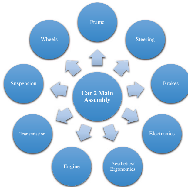
Figure 1.3: Diagram showing the first level break down of the sub-assemblies of Car 2
