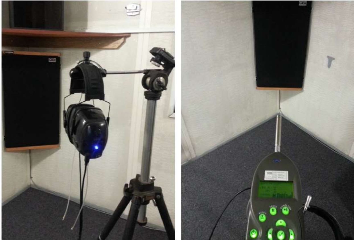
Figure 1. KUDUwave and Sound Level Meter setup during MPANL [ANSI S3.1 (1999(R2013))] measurements
