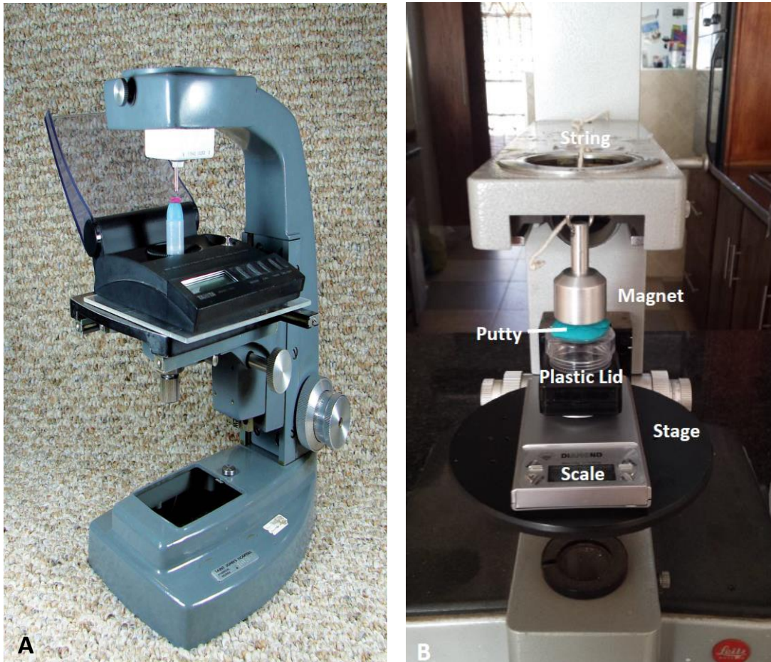
Figure 70. Apparatus used to measure magnetic susceptibility. A: the apparatus used by Hoover et al. (2008). B: the apparatus used in this thesis.
