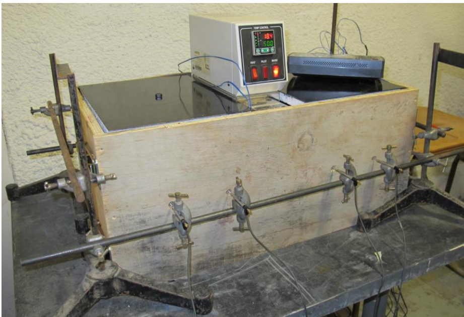
Figure 3.7 Measurement setup with closed box and mounted LVDTs
