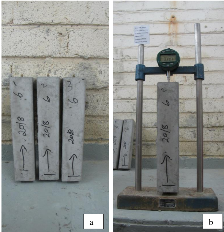
Figure 3.4 Photos of a) orientation of stored samples and b) rig and dial gauge used to measure total long-term deformation
