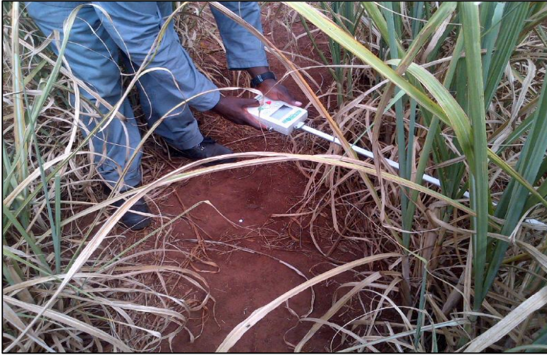
Figure 3.8 Ceptometer (LP-80 AccuPAR- Decagon Devices) taking below canopy PAR readings
