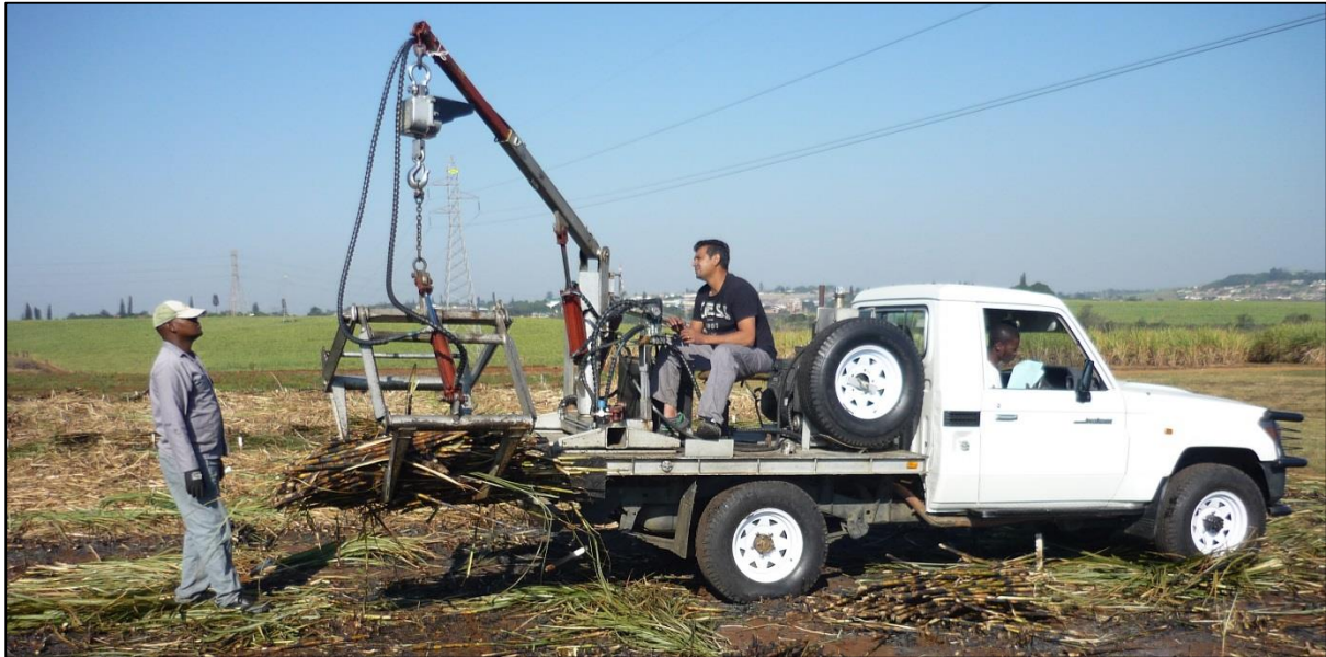
Figure 3.9 Weighing operation done using a weighing pickup with a mechanical grab equipped with a load cell.
