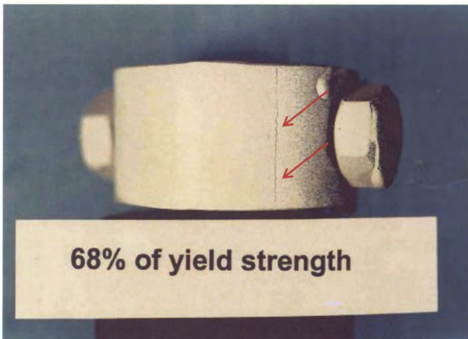
Figure B-4. Magnetic particle test on the specimen stressed to 68% of the yield strength exposed to leaner gas by-product water for 1,000 hours, showing surface cracks.
