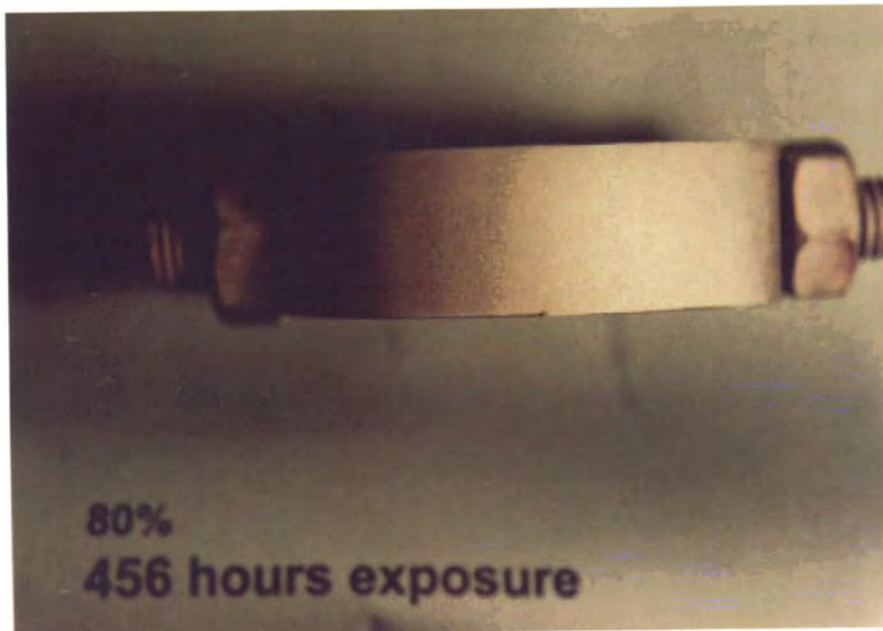
Figure D-3. Magnetic particle test on the specimen stressed to 80% of the yield strength exposed to richer gas by-product water for 456 hours, showing no sign of cracks.
