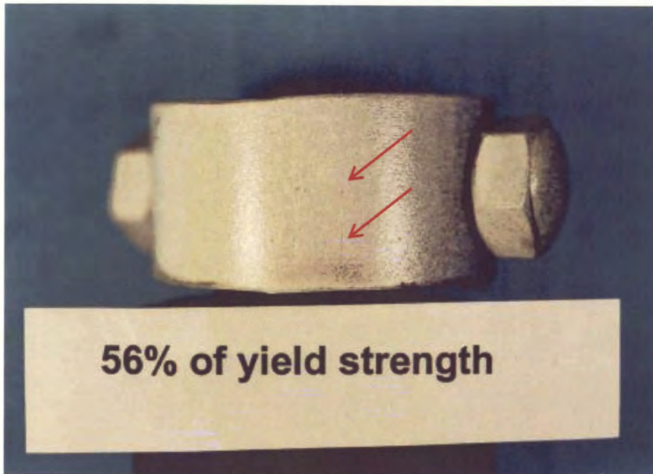
Figure B-5. Magnetic particle test on the specimen stressed to 56% of the yield strength exposed to leaner gas by-product water for 1,000 hours, showing surface cracks.
