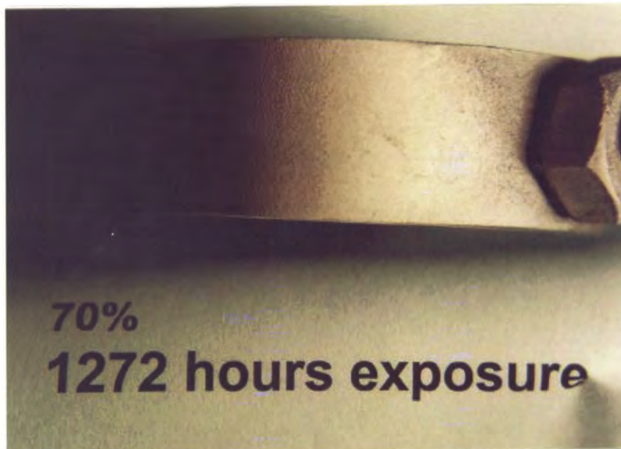
Figure D-22. Magnetic particle test on the specimen stressed to 70% of the yield strength exposed to richer gas by-product water for 1,272 hours, showing no surface cracks.
