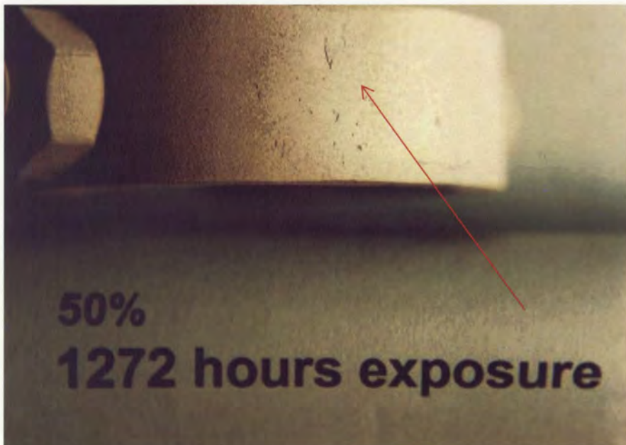
Figure D-24. Magnetic particle test on the specimen stressed to 50% of the yield strength exposed to richer gas by-product water for 1,272 hours, showing surface cracks.
