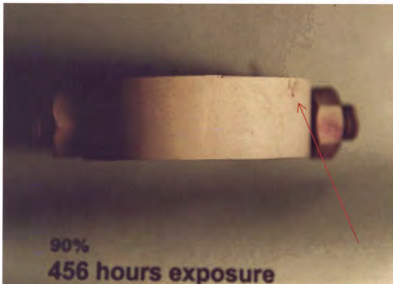
Figure D-2. Magnetic particle test on the specimen stressed to 90% of the yield strength exposed to rich gas by-product water for 456 hours, showing slight evidence of cracking.
