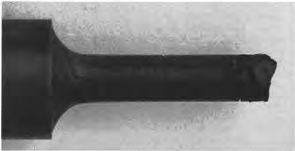
Figure 5-4. An example of a sample after fracture as a result of the cyclic stress conditions, in a CO/CO 2 /H 2 O environment after it failed with R = 0.348 and \sigma_{max} = 147.2 .
