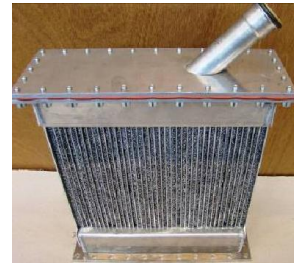
Figure 5 Cooler configuration, used to characterise thermo-hydraulic performance of different aluminum foams
