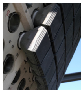
Figure 7: State of the art ceramic receiver modules in the 3MW test receiver.
