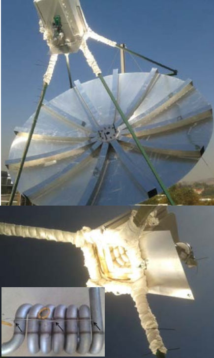
Figure 1 Experimental setup of parabolic dish and tubular receiver [4]
