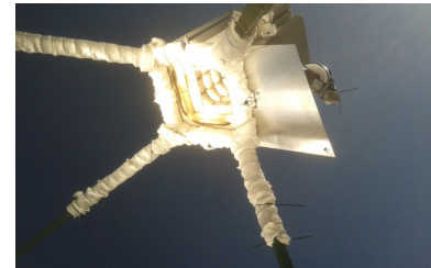
Figure 7 The solar cavity receiver viewed from the bottom.
