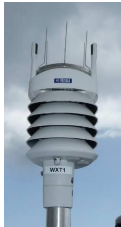
Figure 5 The 6-in-1 WXT520 from VAISALA for weather monitoring
