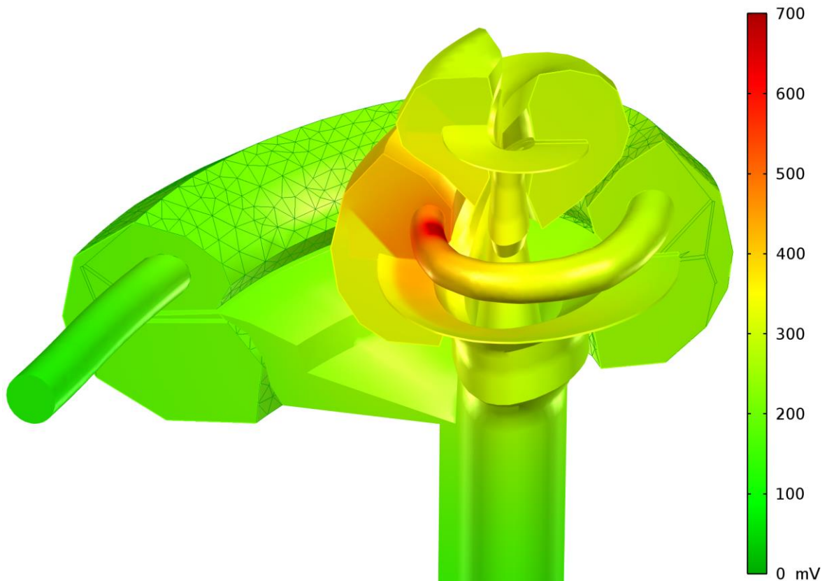
Figure 3.10. Comsol Multiphysics prediction of the electric potential (in mV) in the cochlear model induced by stimulating an electrode at the apical end of the electrode array with a current of 1 mA using monopolar stimulation
