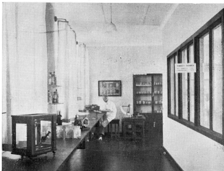
A corner in one of the Wool Research Laboratories showing on the right-hand side the continuous glazing to the Constant Humidity chamber. By means of an air-conditioning plant the air in this chamber is accurately kept at 65% relative humidity and 70° Fahrenheit.
