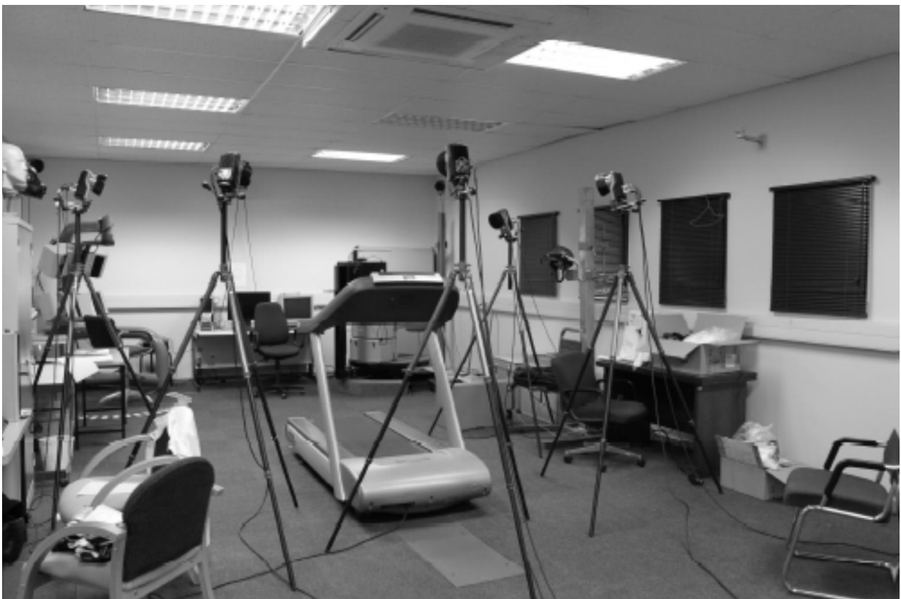
Figure 3.5: Laboratory set-up for each testing session; treadmill positioned centrally with eight cameras positioned around the treadmill.
