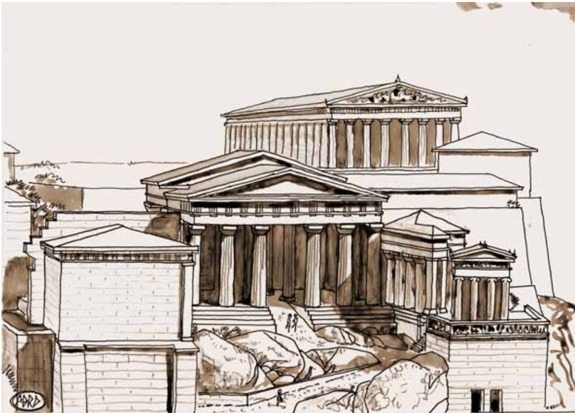
Figure 7 The exterior of the Propylaea, the gateway to the Athenian Acropolis, resembles an incomplete Doric temple that has been purposely fragmented and blemished.
