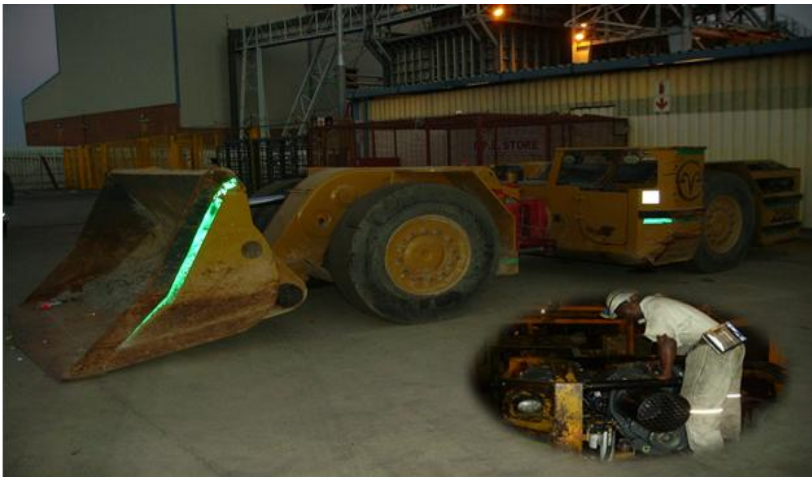
Figure 4-1 LHD vehicle used underground showing the size of the diesel powered engine next to a mine worker (Photographed by G. Geldenhuys)
