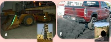
Fig. 1 Sources of DPM: (A) Load haul dump (LHD) vehicle and (B) diesel powered vehicle.
