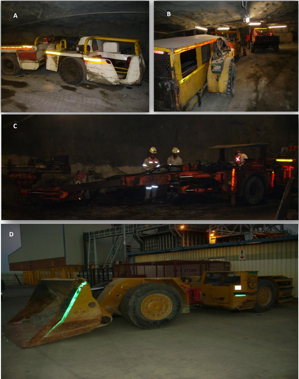
Figure 2-2 Trackless mining vehicles with diesel combustion engines used underground: utility vehicles (A&B), drill rig (C) and a LHD (D) (Photographed by G. Geldenhuys).
