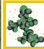
Fig. 7 The physico-chemical composition and structure of DPM (adapted by Maricq, 2007). Green portion represents adsorbed hydrocarbons on the soot.
