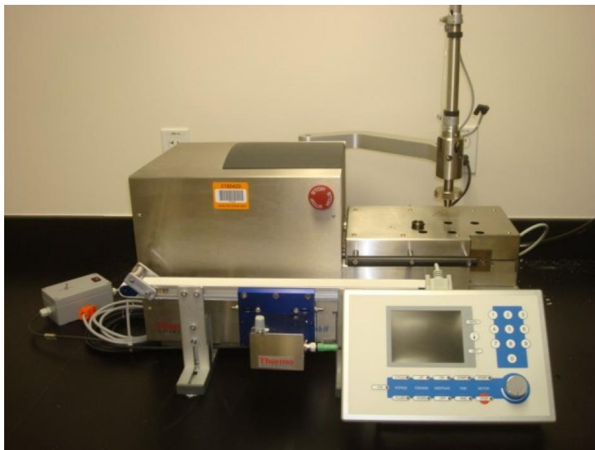
Figure 18: Thermo Scientific Micro Twin Screw Extruder, Sample size = 5g
