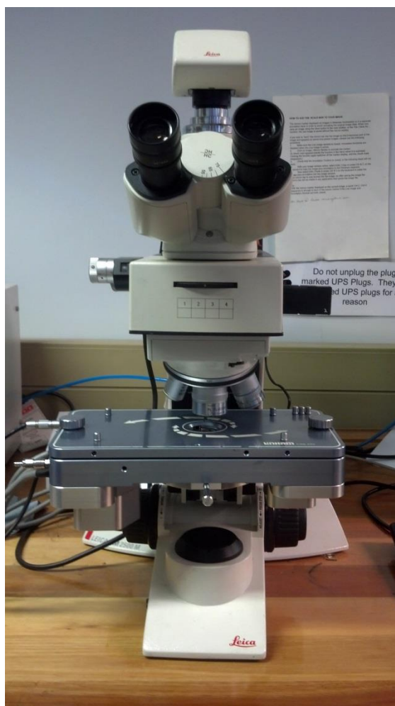
Figure 25: Leica DM2500M optical microscope equipped with Leica DFC420 video camera
