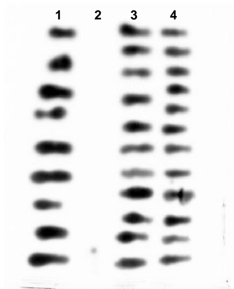
Figure 3.8: Fluorescein-5-EX N-hydroxysuccinimide ester (NHS-fluorescein) glycine conjugate applied to a Stain-Free gel in the absence of protein demonstrates visualisation when the gel is scanned on a Stain-Free Sample Tray. Glycine NHS-fluorescein conjugate (10 mg/ml NHS-fluorescein in DMSO with 1 mg/ml glycine) was pipetted directly onto an exposed Stain-Free gel. Lanes 1, 3 and 4 contained bands made up from volumes of 4 \mu l, 2 \mu l and 1 \mu l of NHS-fluorescein glycine conjugate respectively.
