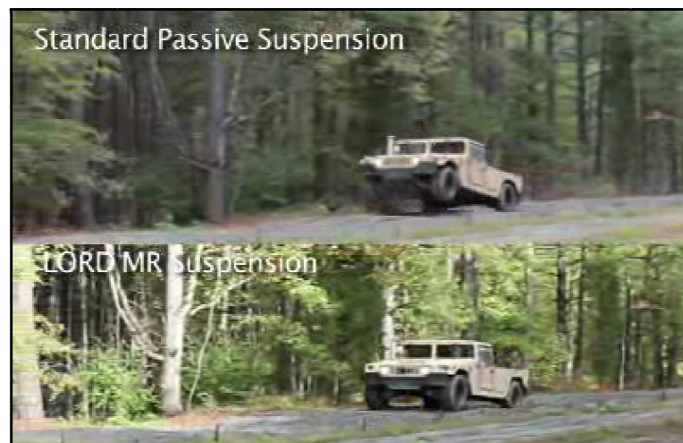
Figure 13: Comparison between the standard damper and MR damper on a HMMWV (Lord.com, 2013)
