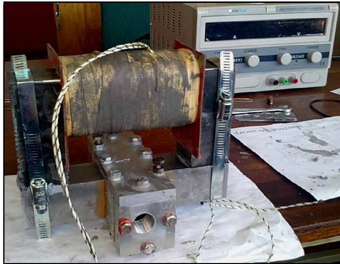
Figure 32: Complete assembled MR valve
