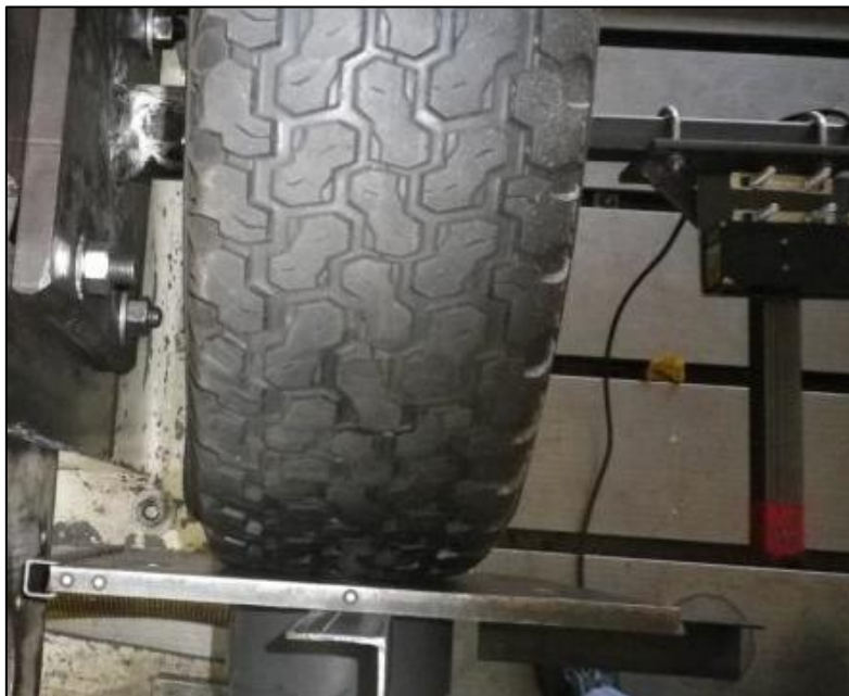
Figure 5.2: Experimental setup for tyre stiffness and cleat tests (seen from above)
