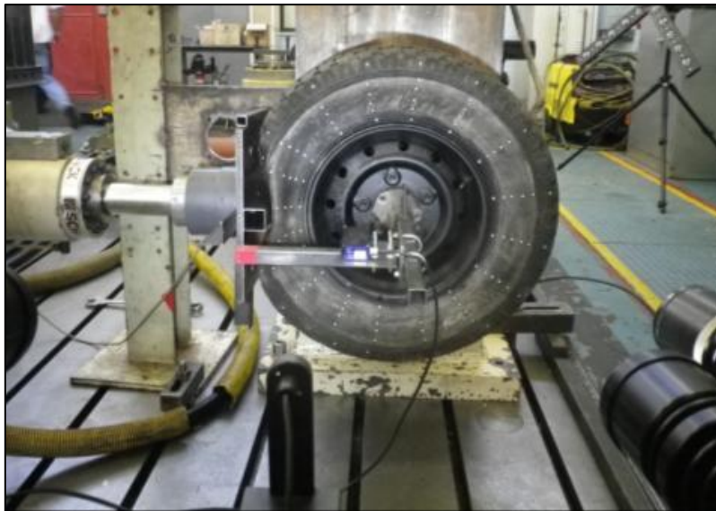
Figure 5.1: Experimental setup for tyre stiffness and cleat tests (side view of tyre) – 51mmx51mm cleat lined up laterally
