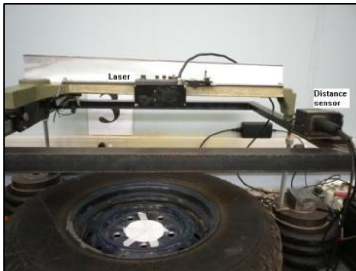
Figure 3.18: Laser profile measurement of the tyre - experimental setup
