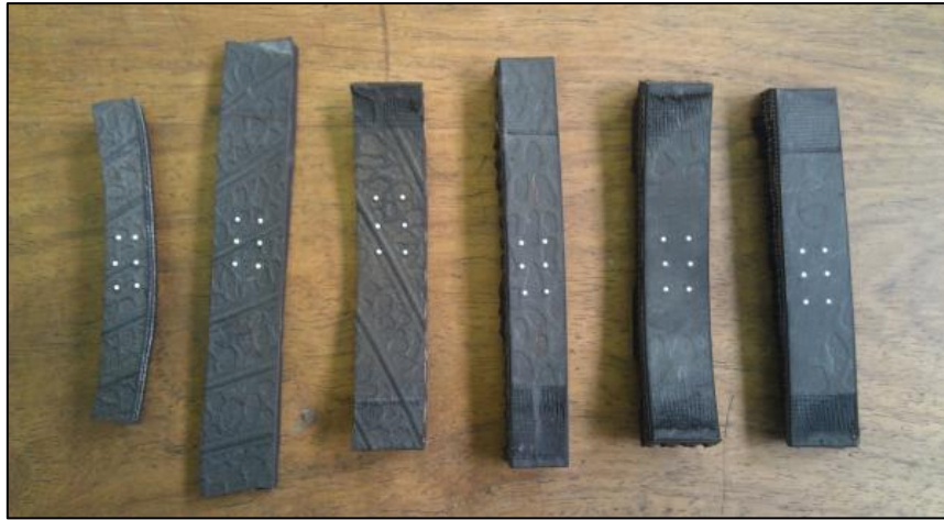
Figure 3.9: Sections cut from the tyre for tensile testing. From left to right, Apex, Sidewall (circumferential), Sidewall (radial), Tread (longitudinal), Tread (lateral), Tread (diagonal)
