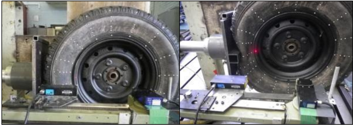
Figure 5.9: Tyre deformation measured using two lasers.
