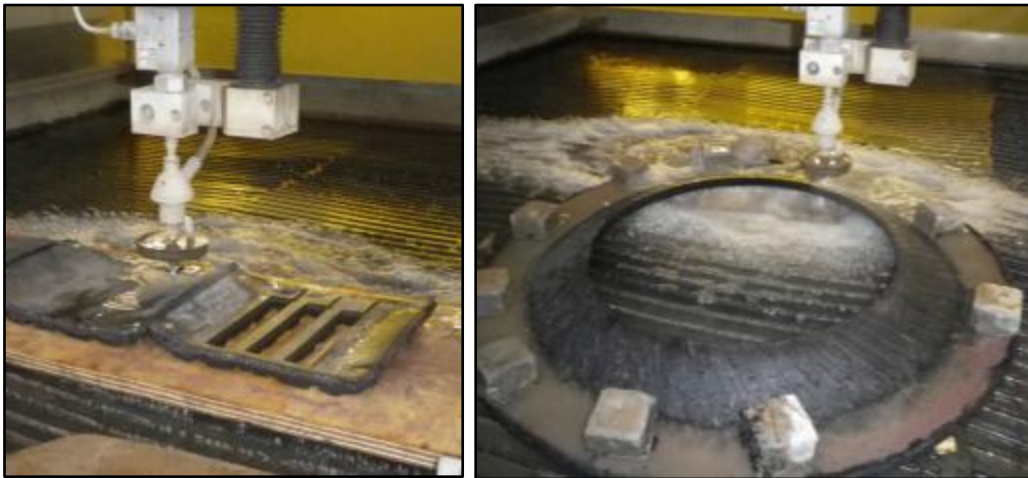
Figure 3.6: Segments of the tread and sidewall being cut using a water jet cutting machine
