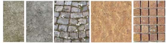
Coral stone and cement composite pavers
