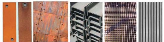
Steel profiles and sheeting reused for construction.
