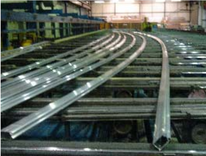
Figure 1 Warped aluminium extrusions subsequent to a spray quenching.
