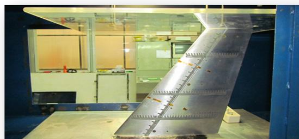
Figure 3- The model with hot film sensors in the test section
