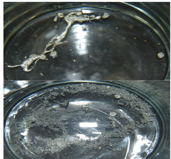
Figure 5 Demonstration of tailored insensitivity with tin melts exposed to variable amplitude shock pulses from detonation of a submerged electrical bridgewire. The top and bottom photos correspond to capacitor energies of ~25 J and 32 J respectively.
