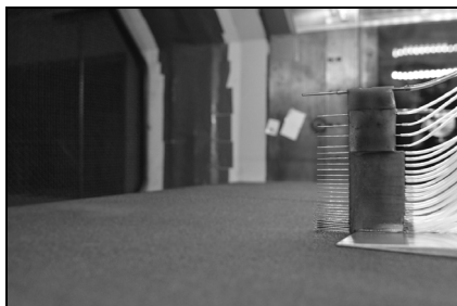
Figure 3 The multiple Pitot rake
