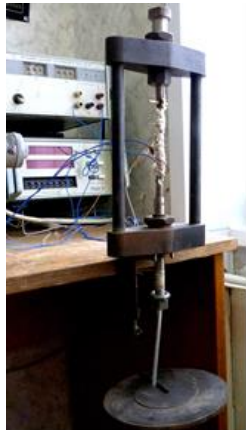
Figure 5 The device for loading of the heat conductor by tensile load
