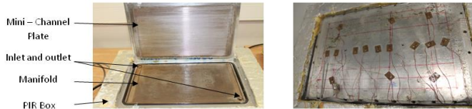
Figure 2 (a) Test Rig (b) Thermocouple arrangement on Plate
