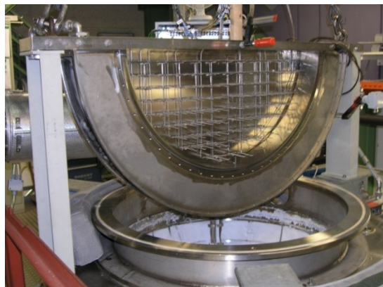
Figure 2 LIVE-2D test vessel with side walls (top) and with the view of heaters (bottom)
