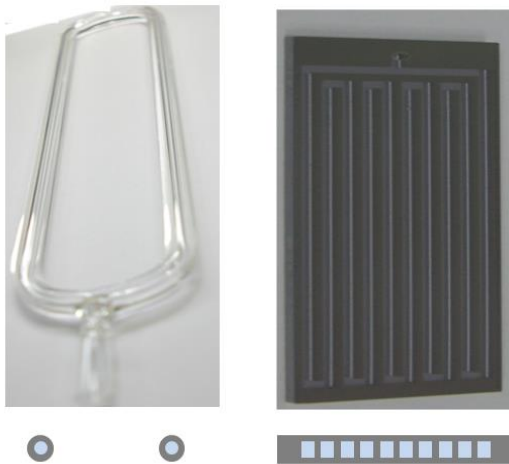
Figure 3 Tubular PHP and flat plate PHP
