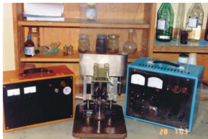
Figure 2. The installation for synthesis of nanocarbon structures and Me-carbon composites in the liquid phase
