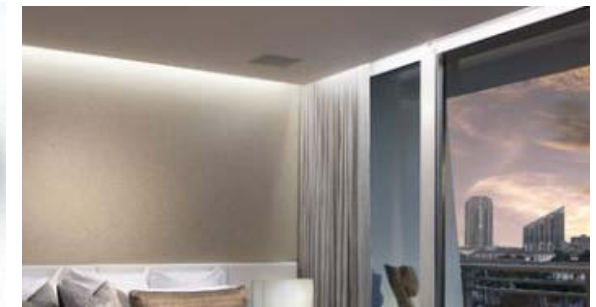
Figure 6.12 Cove lighting effect (Decoist, 2012)
