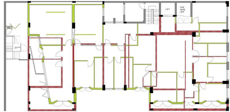
Figure 5.5 First floor demolition plan
