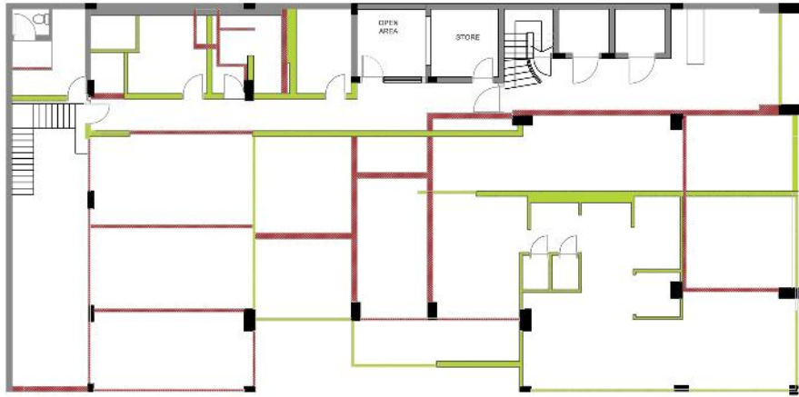
Figure 5.4 Ground floor demolition plan
