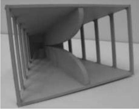
Fig. 1. The 1-18 GHz DRGH antenna [13] used as transfer-standard.
