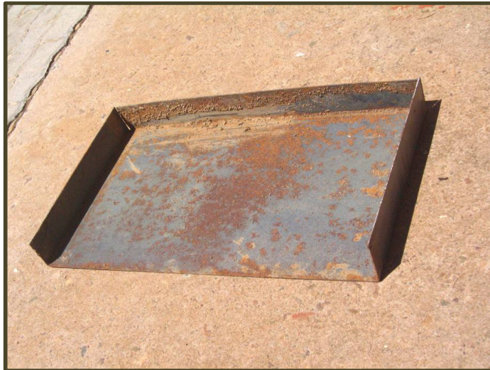
Figure 3.2 Metal tray used to take samples in field
