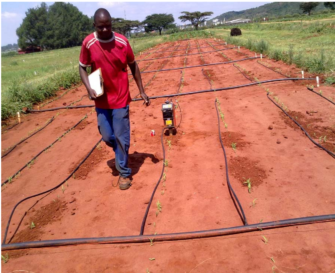
Fig 3.3: Illustration of drip lines layout and the soil water content measuring instrument (Neutron probe) in the sweet sorghum experiment in 2010/2011.
